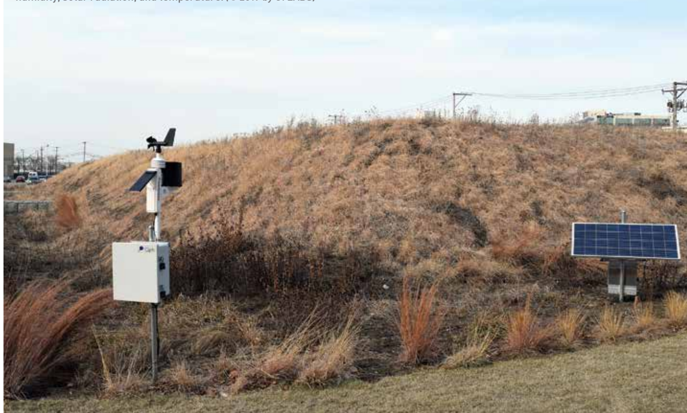
Underground sensors at the UI LABS bioswale in Chicago collect data on soil moisture and groundwater levels, while an above-ground weather station collects data on precipitation, wind, humidity, solar radiation, and temperature. (© 2017 by UI LABS)
