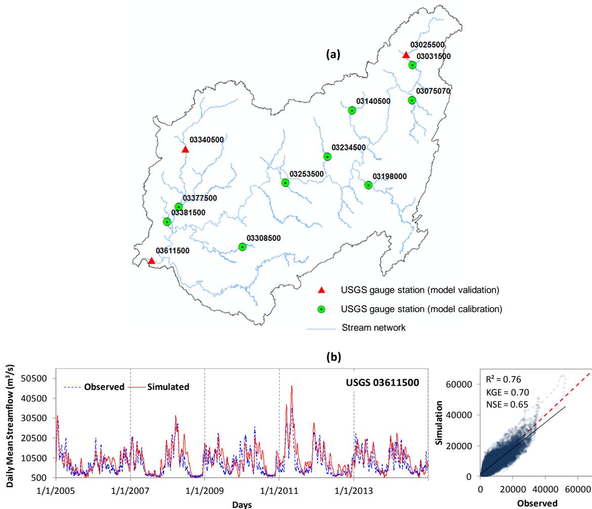
Figure 3. (a) SWAT calibration and validation locations (numbers correspond to respective USGS station IDs); (b) evaluation of model performance at a near-outlet gauge station.
