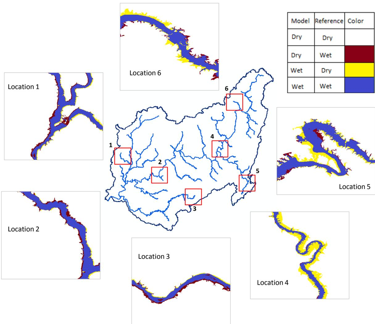
Figure 4. Evaluation of model generated 100 year flood inundation with corresponding FEMA reference.
