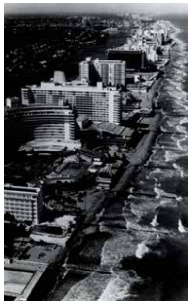
Miami Beach (circa 1972) has no beach along most of its length. Natural beach was lost, in part, due to storms and effects of seawall placement.
